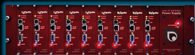
T-Gate blades in a 3U Sub rack with Integrated PSU for 9 gateway cards
